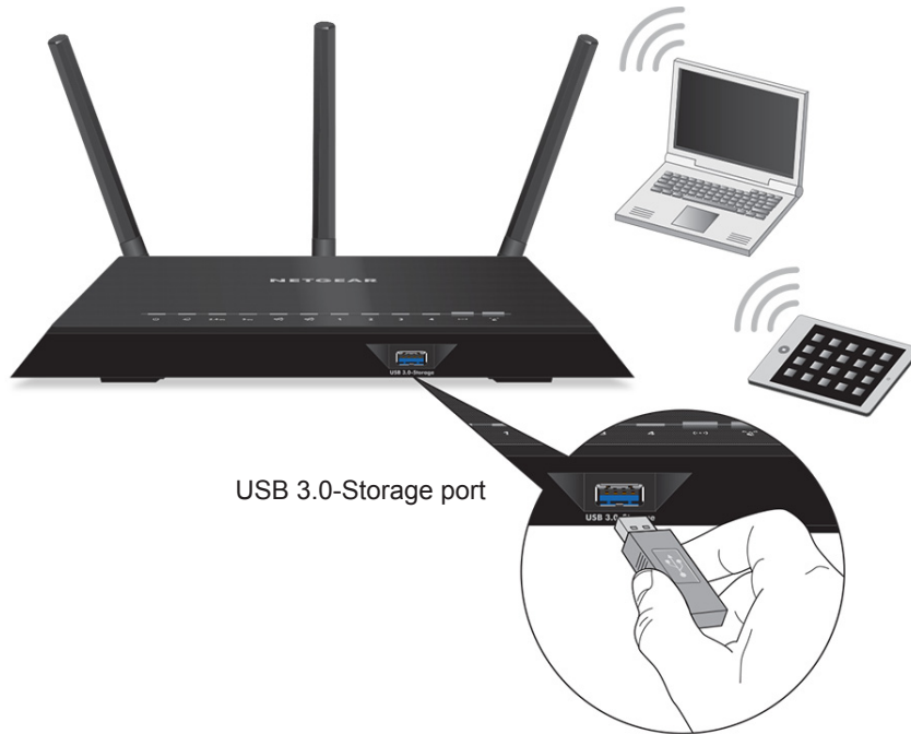
Figure 9. The blue USB 3.0-Storage port on the front of the router provides the fastest access
