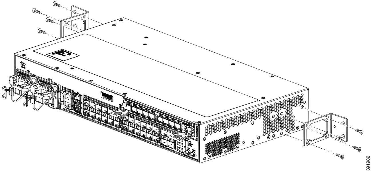
**Figure 3-6** Attaching Mounting Brackets to Cisco ASR-920-24SZ-M, ASR-920-24TZ-M Router for a 300 mm ETSI Rack (Front, Middle, and Rear Positions)
