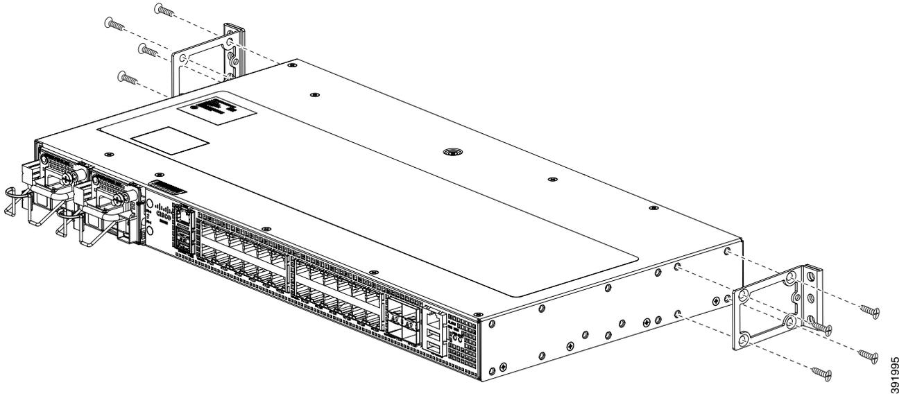
**Figure 3-3** Attaching Mounting Brackets to Cisco ASR-920-24SZ-IM Router for a 23-inch Rack (Front, Middle, and Rear Positions)
