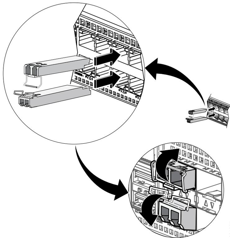
**Figure 3-30** Installing an SFP Module without a Bale-Clasp Latch into an SFP Module Slot on Cisco ASR 920-24SZ-IM, ASR-920-24SZ-M, ASR-920-24TZ-M Router
