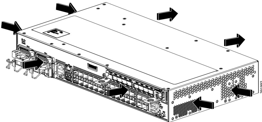
**Figure 2-2** *Air Flow in the Cisco ASR-920-24SZ-M, ASR-920-24TZ-M Router*
