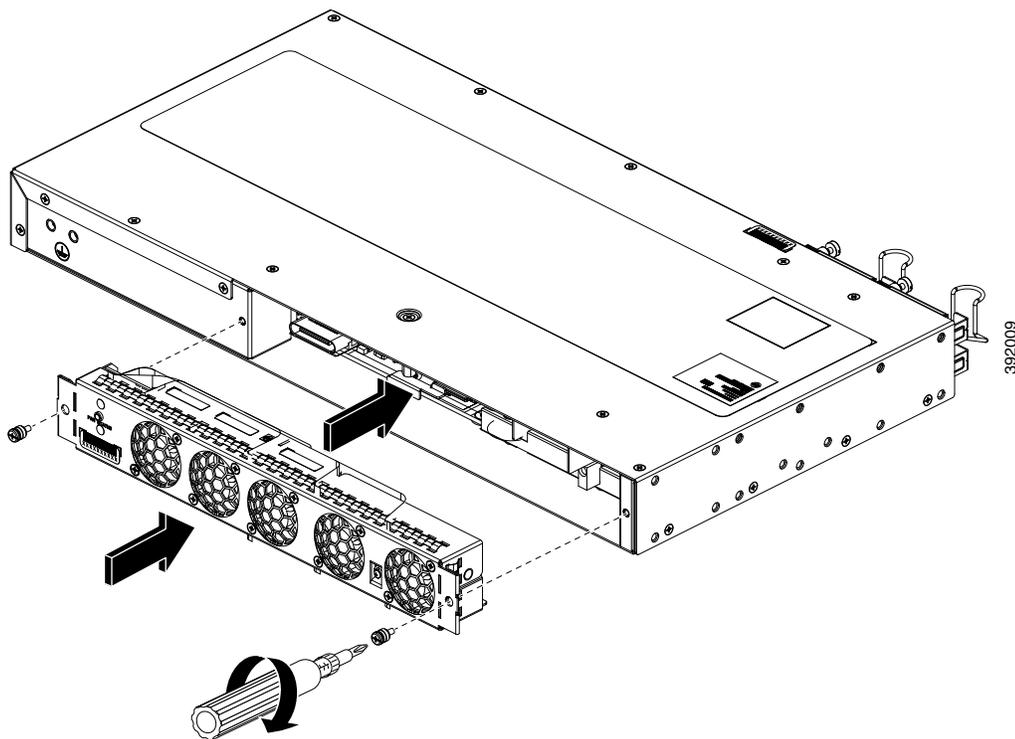
This completes the procedure for installing or replacing the fan tray in a Cisco ASR 920-24SZ-IM, ASR-920-24SZ-M, ASR-920-24TZ-M Router.
