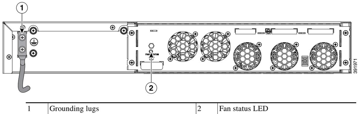
**Figure 3-34 Attaching a Grounding Lug to the Rear of the Cisco ASR-920-24SZ-M, ASR-920-24TZ-M Router**
