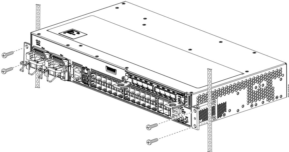
**Figure 3-8** Installing the Cisco ASR-920-24SZ-M, ASR-920-24TZ-M Router in a 19-inch EIA Rack
