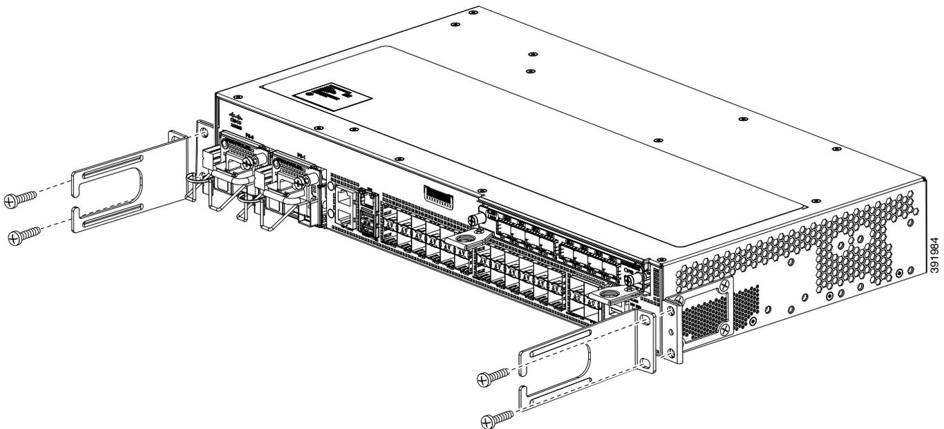
Figure 3-10 Installing the Cable Guides on Cisco ASR-920-24SZ-IM Router (As Per the Standard Kit)
