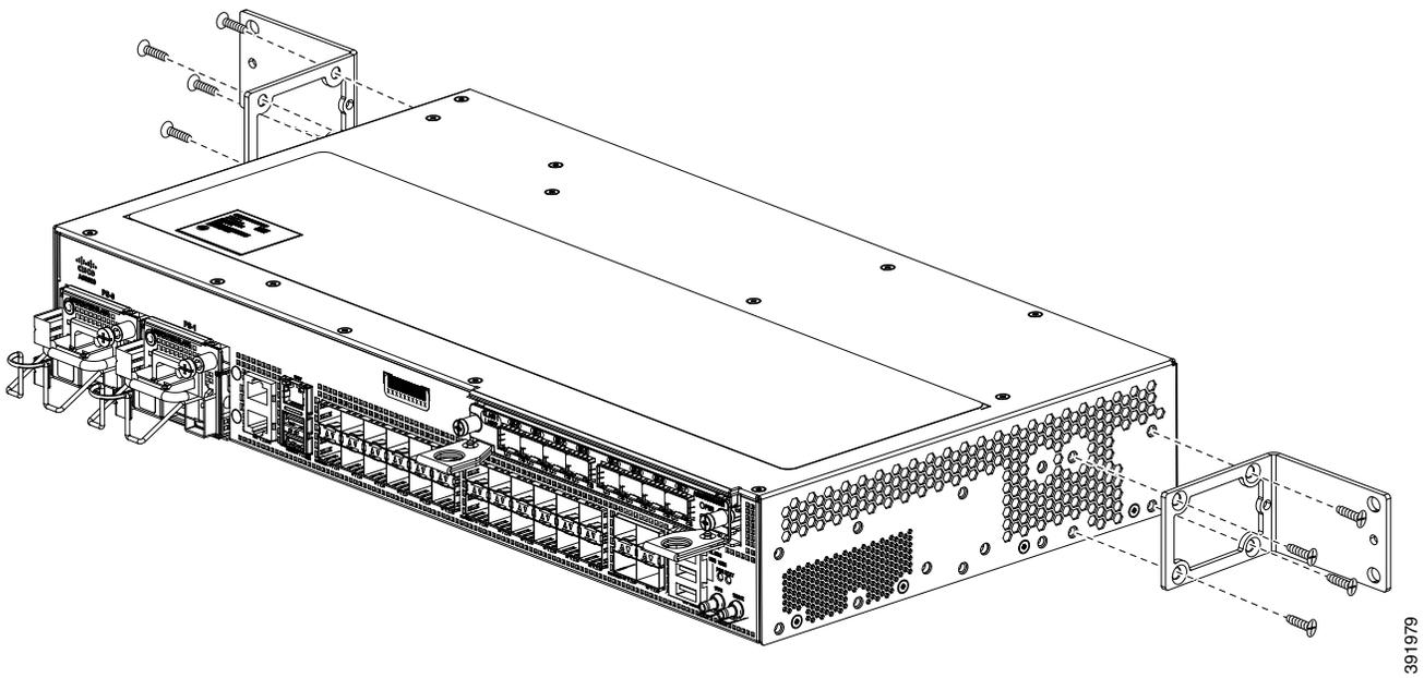
**Figure 3-4** Attaching Mounting Brackets to Cisco ASR-920-24SZ-M, ASR-920-24TZ-M Router for a 23-inch Rack (Front, Middle, and Rear Positions)
