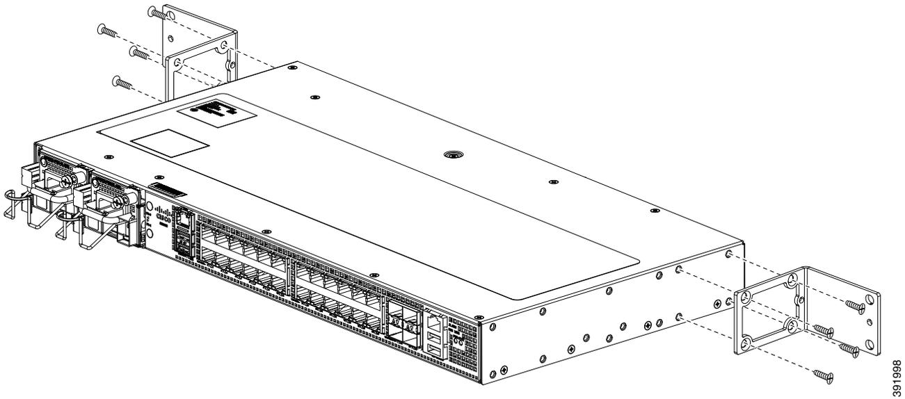
**Figure 3-5** Attaching Mounting Brackets to Cisco ASR-920-24SZ-IM Router for a 300 mm ETSI Rack (Front, Middle, and Rear Positions)
