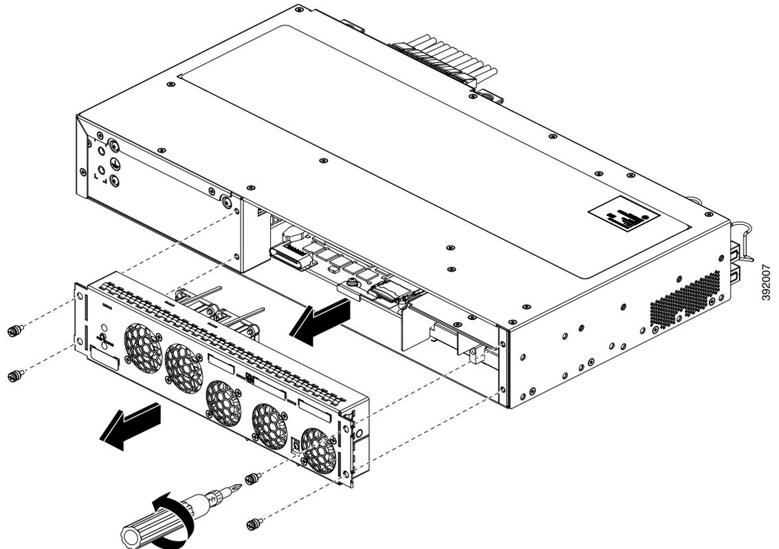
**Figure 3-19** Removing the Fan Tray From Cisco ASR-920-24SZ-M, ASR-920-24TZ-M Router
