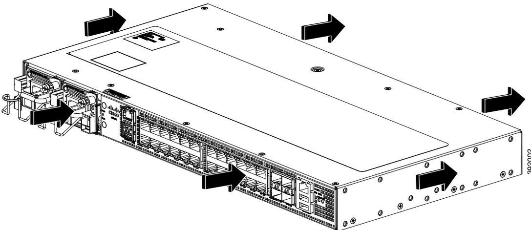
To ensure adequate air flow through the equipment rack, it is recommended that you maintain a minimum clearance distance as mentioned below, at all times.
