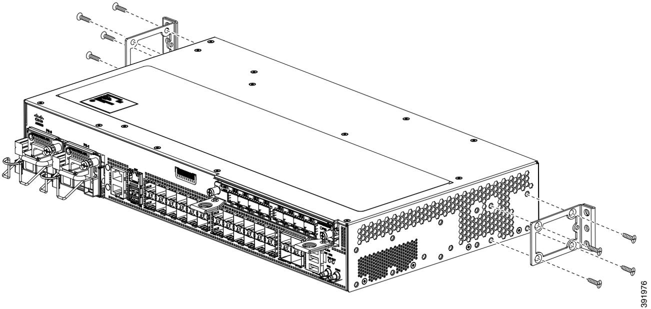
**Figure 3-2** Attaching Mounting Brackets to Cisco ASR-920-24SZ-M, ASR-920-24TZ-M Router for a 19-inch EIA Rack (Front, Middle, and Rear Positions)
