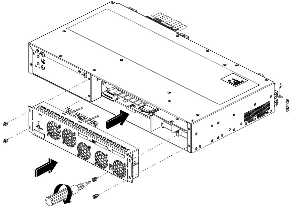
**Figure 3-17** Installing the Fan Tray on Cisco ASR-920-24SZ-M, ASR-920-24TZ-M Router
