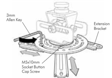
**F.2.** Place the Ceiling Mount Assembly over the Projector and align the centre of the Ceiling Mount with the Centre of Gravity marked previously on the Projector.
