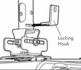
**G.3.** Tighten the Locking Hook with the supplied M8x50mm Socket Cap Screw and the M8 Nyloc Nut.
