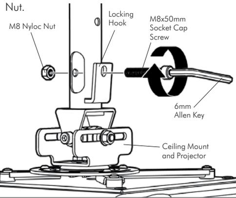
**Tip:** When the projector requires servicing, remove the projector via this easy disconnection point to save time.
