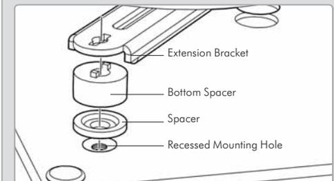
**F.4.** Select the correct Mounting Screws from the Bits Bag and firmly secure the Ceiling Mount Assembly onto your Projector.
