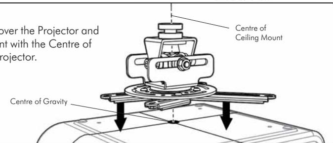
**F.3.** Place the Bottom Spacers in between the Extension Brackets and the Projector, and align the mounting holes as shown below.
