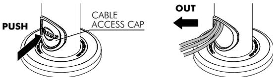
**A.** Push out to remove Cable Access Cap
