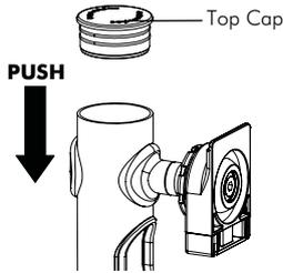
Push down firmly to attach the Top Cap.
