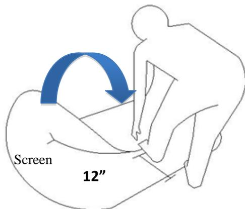
2) While holding the material down with both feet, lean forward and grab the left and right side.
