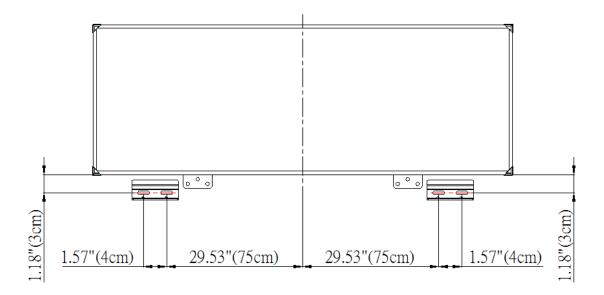
Minimum clearance requirement for pen tray installation diagram
