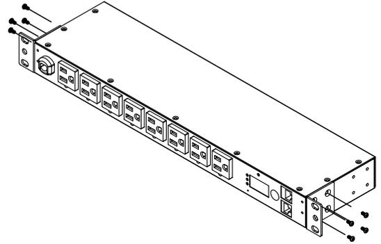
If you plan on attaching the Cord Retention Tray to the PDU, you will need to use the LONG Mounting Brackets (2).
