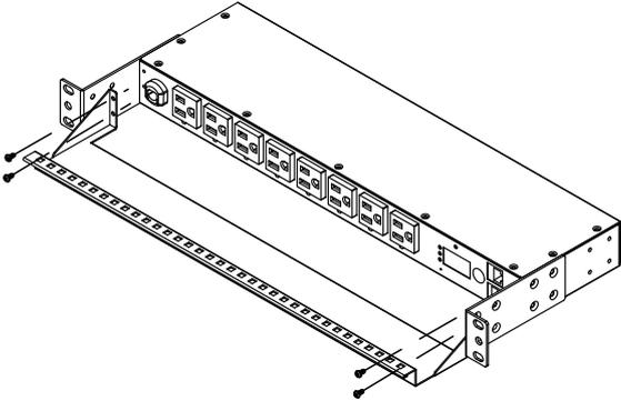
Use the provided Cable Ties to fasten each cord to the Cord Retention Tray.
