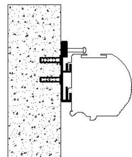
1. Determine where the screen will be installed. Then, measure and mark the distance between the top and bottom screw holes from each **hidden wall mount bracket** (H).
