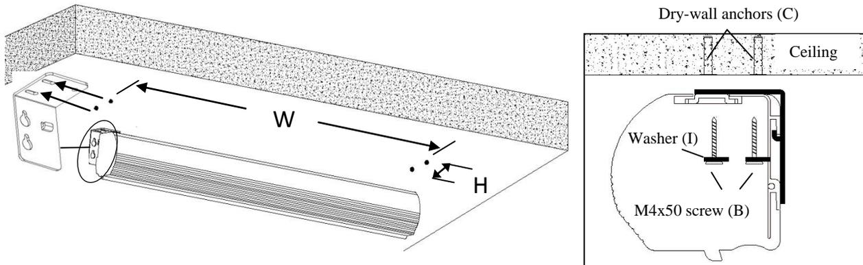
**NOTE: The brackets do not slide. They are designed to attach the end caps only.**
