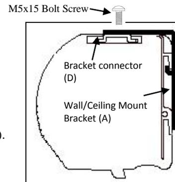
1. Begin by sliding the **bracket connector** (D) all the way to each end of the housing.
