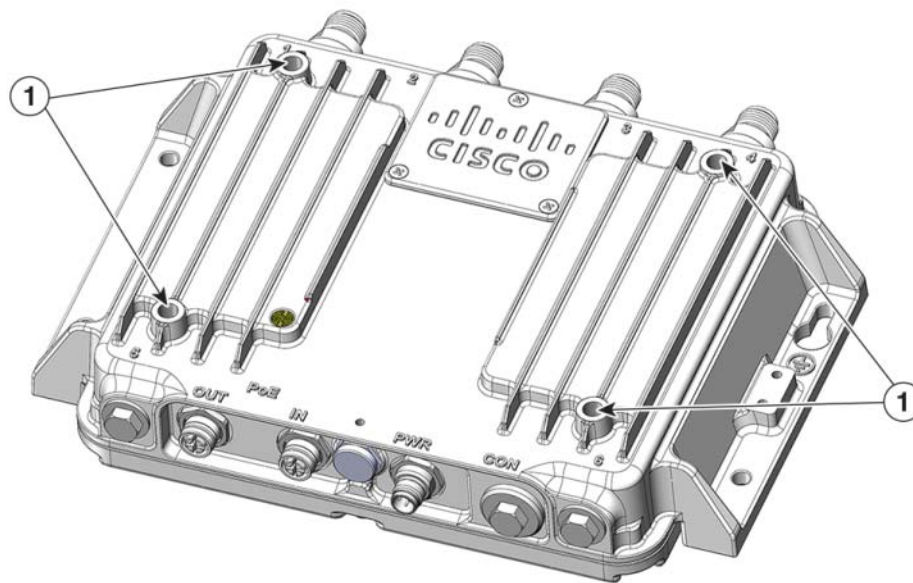
Figure 5 Cisco IW3702 Series Access Point Hard Points
